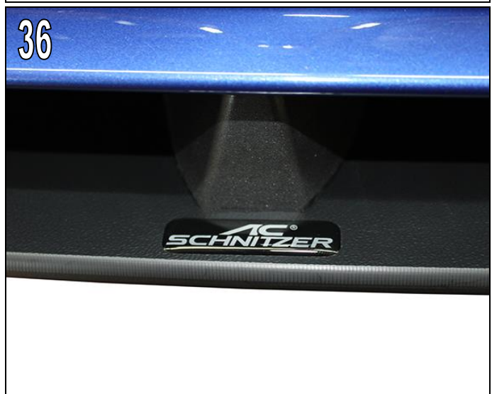
Fig. 36 Affix the AC Schnitzer sticker supplied in the recess provided in the AC Schnitzer front splitter.
