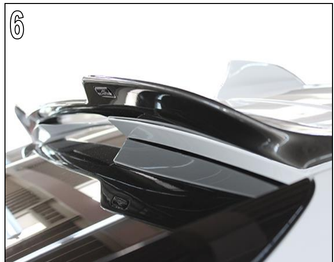
Fig. 5 & 6 The contour of the AC Schnitzer rear roof wing must run parallel to the contour of the tailgate on the right and left.
