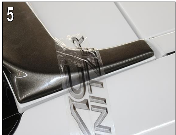
Fig. 4 Place the AC Schnitzer rear roof wing on the vehicle.
