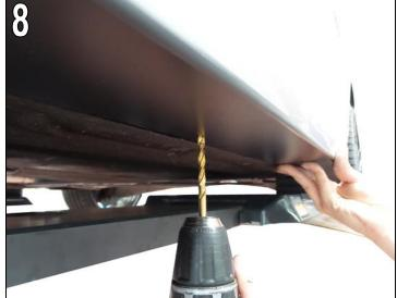
Remove spread rivets at front and rear, and remove the AC Schnitzer side skirt again.
