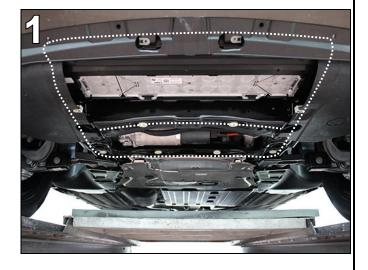
**Fig. 1**Remove the underbody panelling. To do this, loosen all 14 fastening screws. (Picture shows removed underbody panelling).
