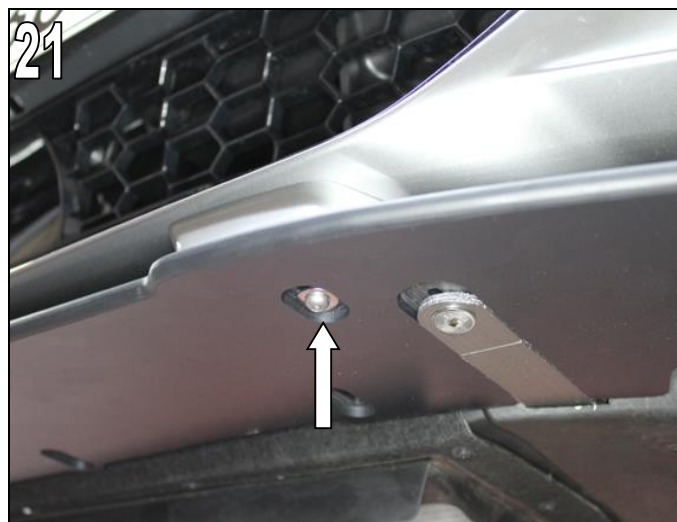
Fig. 21 Secure the AC Schnitzer front splitter to the AC Schnitzer mounting adapter using the cap-head bolts M6x45mm and washers U6.4x18mm supplied.
