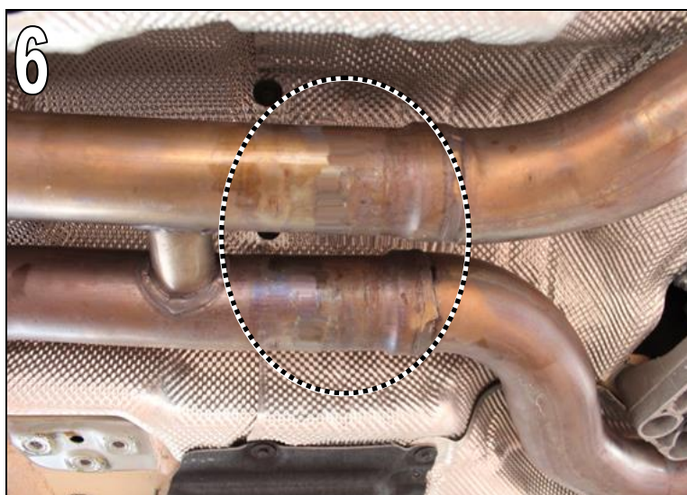
Fig. 6 Make a cutting mark in the part of the exhaust system shown. (in direction of travel – to the front)
