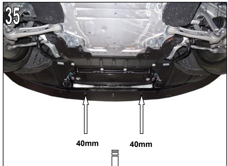
Figs. 35 & 36 Position 40mm spacer sleeve between AC Schnitzer front splitter and standard front skirt as shown.
