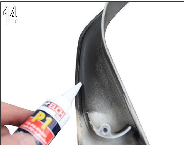
Clean the adhesive surface on the rear skirt insert with the supplied cleaner.
