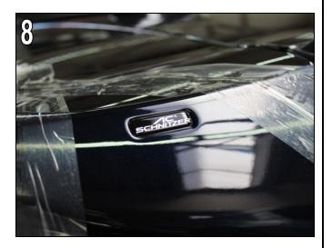
The adhesive drying time is 24 hours. The vehicle can be washed in a car wash after around 48 hours.
