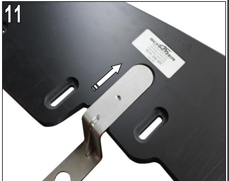
Fig. 11 Lay AC Schnitzer fixing bracket in the AC Schnitzer front splitter as shown.
