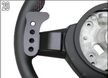
Figs. 20 & 21 Insert AC Schnitzer shift paddle into the steering wheel, and secure using the standard fixing bolt.
