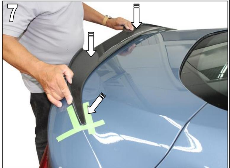
Press on AC Schnitzer carbon rear spoiler firmly.
