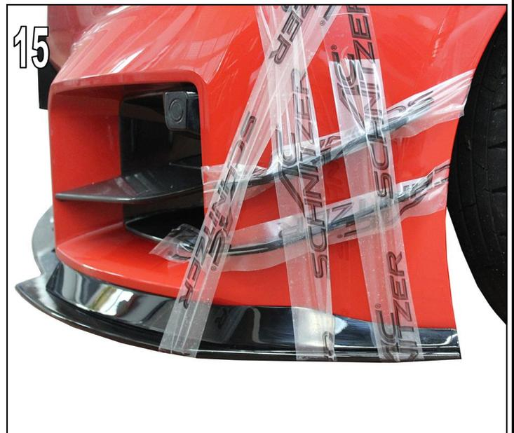
Ensure that the AC Schnitzer front side wings are parallel.
