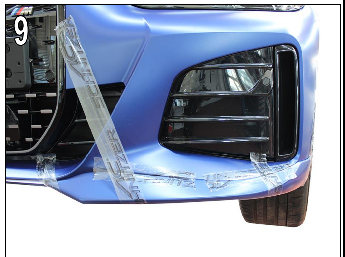
Fig. 9 & 10 Affix the AC Schnitzer front spoiler element with masking tape. If necessary, use AC Schnitzer mounting aids or rebounds as mounting aids.
