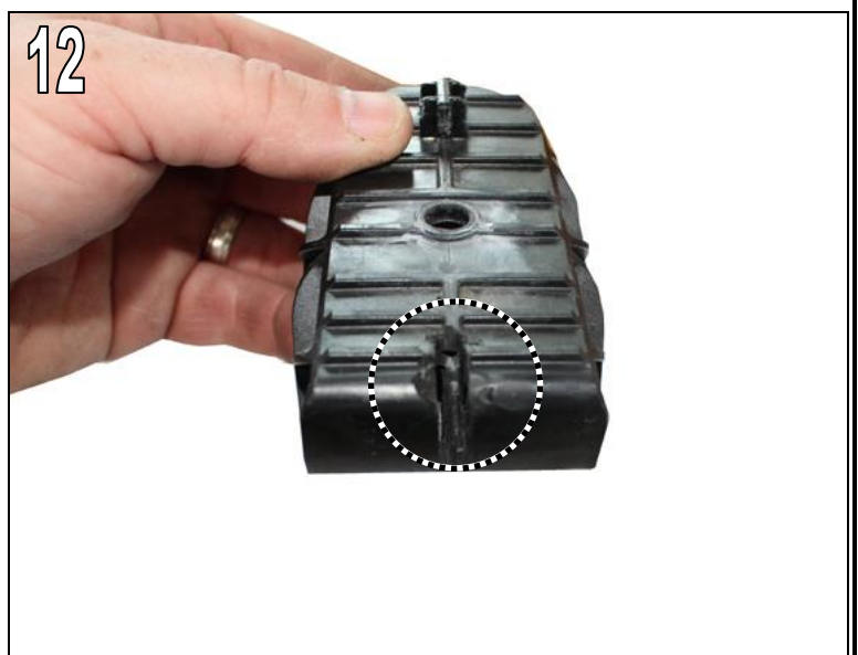
Fig. 12 & 13 Using a suitable tool, mill out the standard bracket at the marking previously applied until the AC Schnitzer fixing bracket fits perfectly and rests on the standard bracket.
