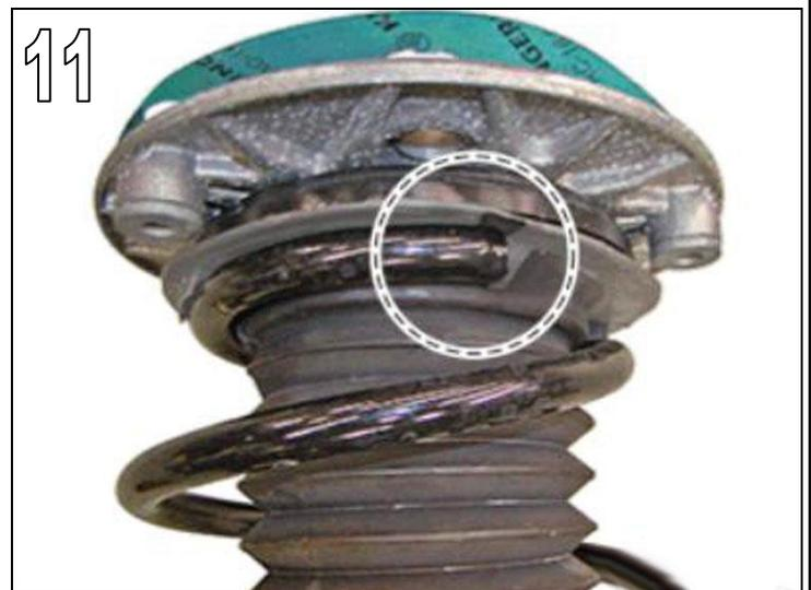
Replace nut and tighten with special tool 33 0 040. Note tightening torque.
