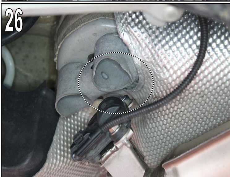
Fig. 26 M4 Cabrio (G83) If necessary: Ensure sufficient clearance from the exhaust flap motor to the torsion strut.
