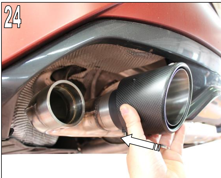
Fig. 24 Push the AC Schnitzer tailpipe carbon sport onto the AC Schnitzer silencer.
