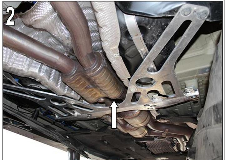
Support the series muffler with a suitable aid.
