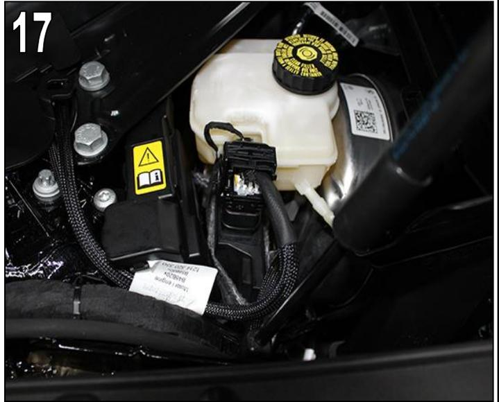
Restore the engine +12 Volt power supply by refitting the cable line to the +12 Volt central point.
